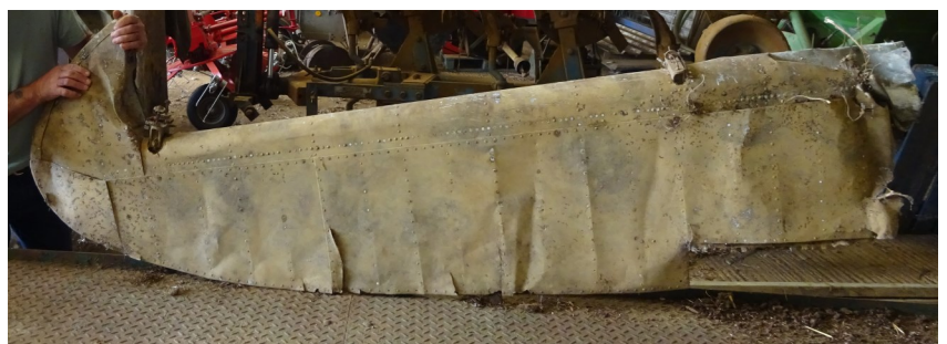
Tail plane section of the De Havilland DH98 Mosquito T MK III
